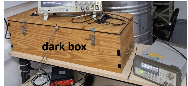
C-Arapuca's pulse with a 395 nm UV LED in the dark box.
