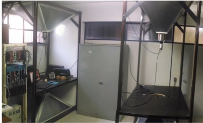
Muon telescope with four plastic scintillators
