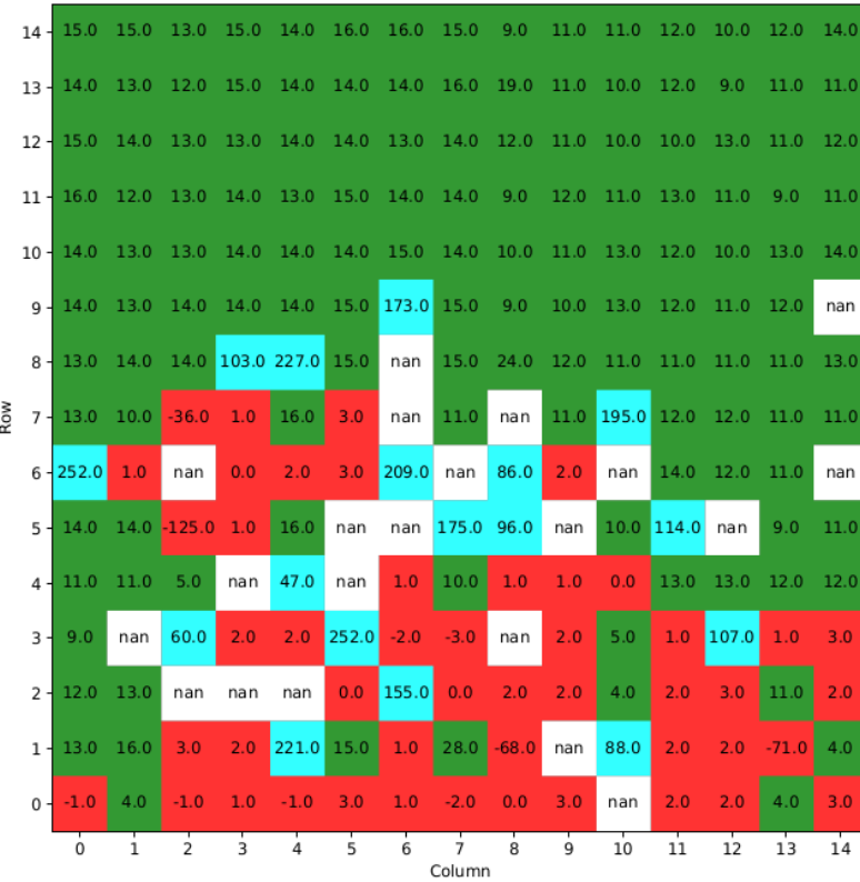
ASIC 0 - 48 disconnected and 17 bad
