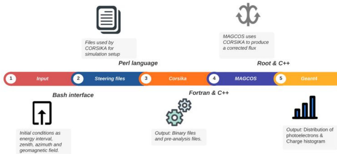
Fig. 2 As the simulation evolves, the different ARTI modules call CORSIKA, MAGCOS, or Geant4 to accurately calculate the signal flux at the detector expected by the integrated cosmic ray flux. The simulation moves forward as a sequence: the results from one steps are used as inputs for the next one
